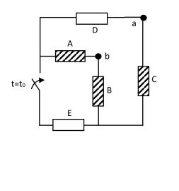
2) Define polarities as you wish, if V<sub>E</sub> = # kV, V<sub>D</sub> = 1.5\*# kV, V<sub>B</sub> = 0.75V<sub>E</sub>, a) Build the potential diagram for the circuit ∀t, b) Using that diagram compute V<sub>ab</sub> for t<t<sub>0</sub>. c) compute also V<sub>s</sub> for t>t<sub>0</sub>.
