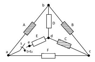
Define polarities as you wish, if V<sub>A</sub> = # kV, V<sub>B</sub> = 1.5\*# kV, V<sub>C</sub> = 0.75V<sub>A</sub>, a) Build the potential diagram for the circuit ∀t, b) Using that diagram compute V<sub>E</sub> ∀t. c) compute V<sub>s</sub> ∀t.
