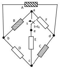
2) If  $V_C = -3V_B = 2V_F = \# kV$ , a) plot the potential diagram for the circuit  $\forall t. b$ ) Using the potential diagram compute V<sub>be</sub>. Polarities and reference node will be assigned by the professor during the test.
